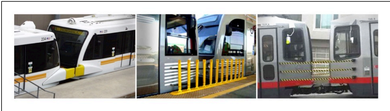
Figure 4-7 – Between-Car Barriers in Light Rail Applications
